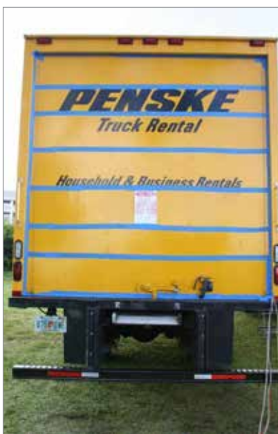
B. Example of trailer using tape to seal gaps on doors and other openings.
