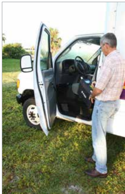
Leak testing after introduction on tape-and-seal applications can identify areas where additional sealing is needed and can improve fumigant confinement.
