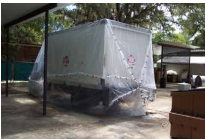
A. Example of tarping an entire trailer by driving it on top of the tarp and then wrapping it.
