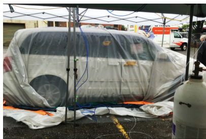
Fumigant was applied to this van through a high-density polyethylene introduction hose.
