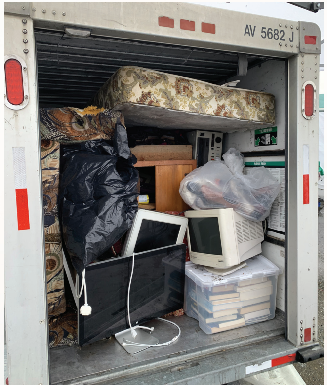
Test trailers were filled to 85 percent capacity with books, furniture and other household items to mimic cluttered living spaces. (All treatment photos courtesy of Virginia Tech)
