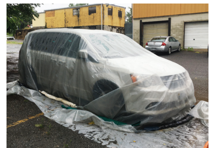
A polyethylene sheet served as a tarp that was sealed to the ground around this van.
